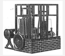
This logistical challenge was expensive and time consuming, so Gorrie started experimenting with the concept of artificial cooling. In 1851 he designed and patented a machine that created ice using a compressor powered by a horse, water, wind driven sails or steam.
